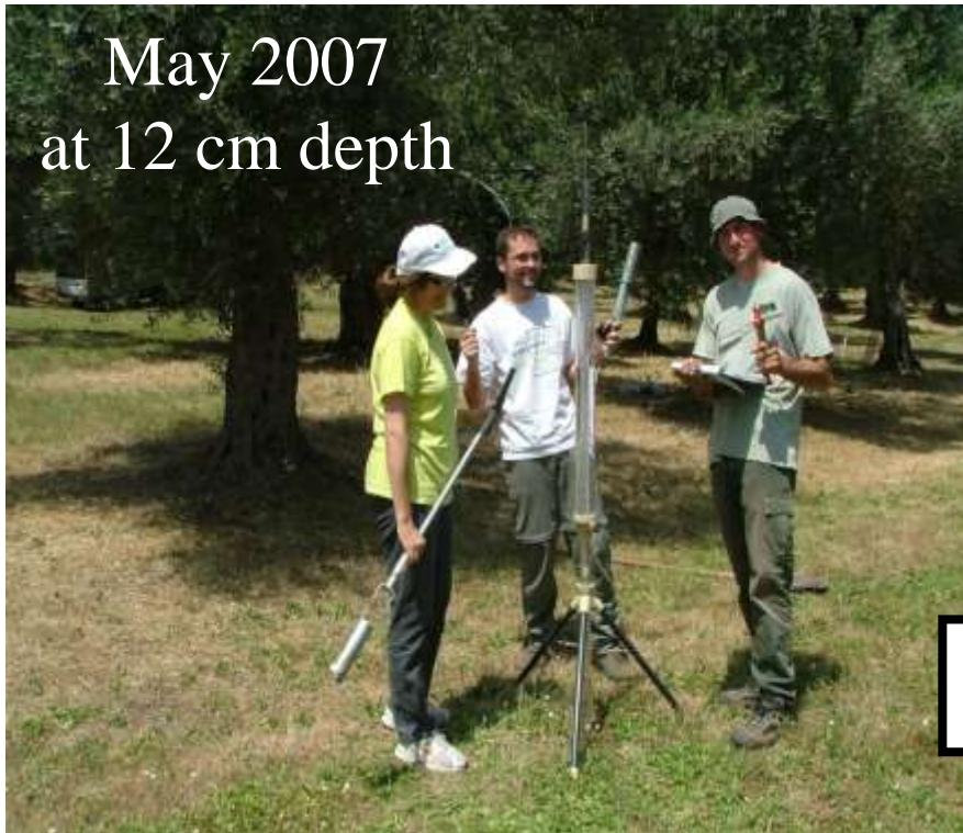
Evaluation of the vertical water flux (using a plastic tube as confined well)
