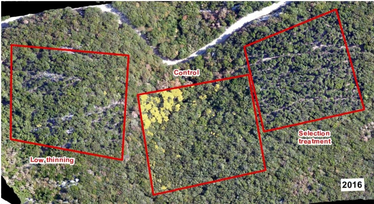
Figure 3. Limits of the Requesens pilot experience (red polygons) over the aerial image of 2016. Yellow polygons refer to decoloured crowns, identified with the supervised classification of ArcGIS.
